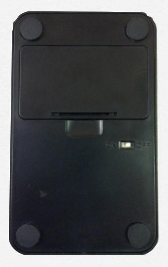
Step 1 Open the battery cover, put two AA battery. Turn on the power button to "on". Blue LED could blink around 5 seconds.
